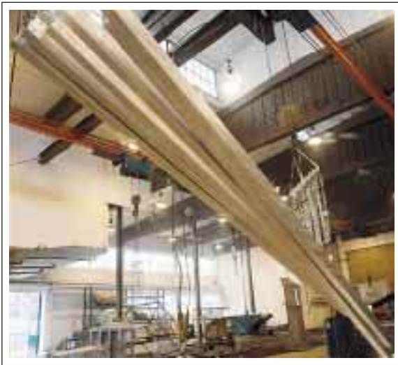
Large lifting height facilitates good runoff from the goods
