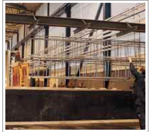
The goods is by hand suspended on special fixtures. From that moment the operation is computer controlled.
