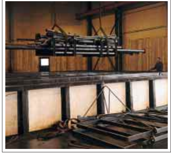
The goods is degreased by means of environment friendly tensides. It is then pickled in a couple of pickle baths before it is transferred to the zinc bath
