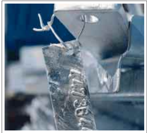
Distinct tagging facilitates identification after the galvanizing.
