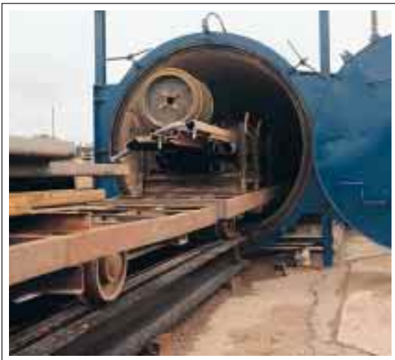
If the goods is covered with paint or varnish, this coating is removed by burnoff in an oven (Ø 2,0 x 9,5 m).
